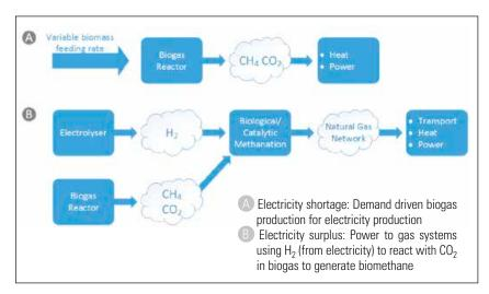
Figure 2: The role of biogas in the smart grid.
