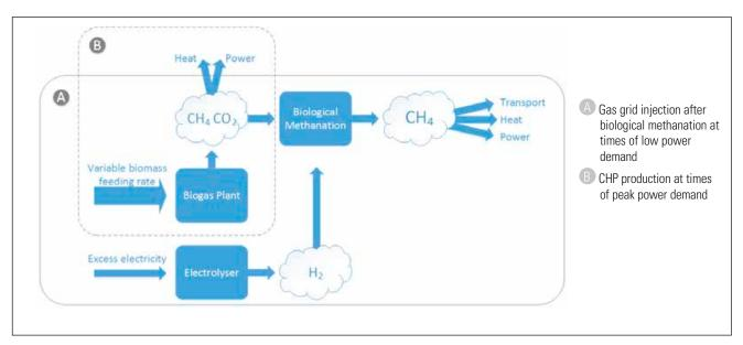
Figure 12: Co-location of CHP and biological methanation (from Ahern et al., 2015)
