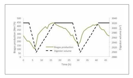
**Figure 7:** Biogas production and feed injection during a 48 hour period at Sobacken biogas plant in Borås. (Source: Borås Energi och Miljö)
