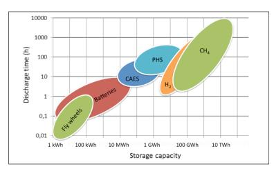
**Figure 1:** Comparison of various energy storage systems with respect to discharge time and storage capacity (modified from Specht et al., 2011).
