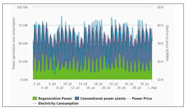
**Figure 3.** Generation and consumption of electricity in Germany in July 2014, also showing actual electricity consumption and electricity prices (Note: Regenerative Power includes renewable electricity from solar, wind, biomass and water) (Source: Agora Energiewende).
