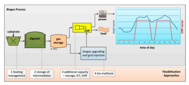
Figure 6: Approaches for biogas-based demand driven power production (Szarka et al, 2013)
