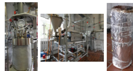
Figure 1: Reactors: HTC (left), pyrolysis-N 2 (middle), pyrolysis-air (right).
