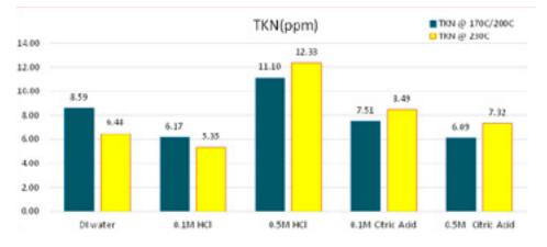
Figure 1 TKN in the aqueous phase at low and high temperature with and without acid addition. Low temperature is 200 °C for DI water and 170 °C for all other cases Pierpaolo Modugno, Queen Mary University of London
