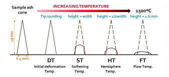
Figure 1. Schematic of the AFTs determination procedure.
