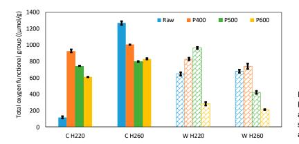
Figure 1. Total oxygen functional groups on raw, hydrochars, and thermally activated hydrochars at various temperatures. Note: C/W H220 stands for cellulose/wood hydrochar prepared at 220 °C
