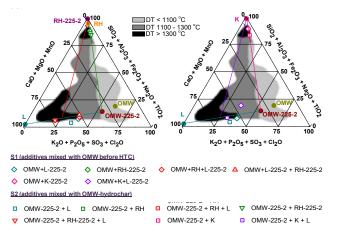
Figure 2. Multicomponent phase diagram illustrating the DT of the samples as a function of ash composition.
