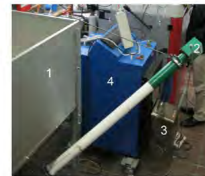
Pellet burner with pellet storage and automated feeding system. 1: Storage for wood pellets, 2: Electrical feeding system, 3: Pellet burner with control unit and housing, 4: Burner, adapted for experimental use, originally a simple wood burner.
