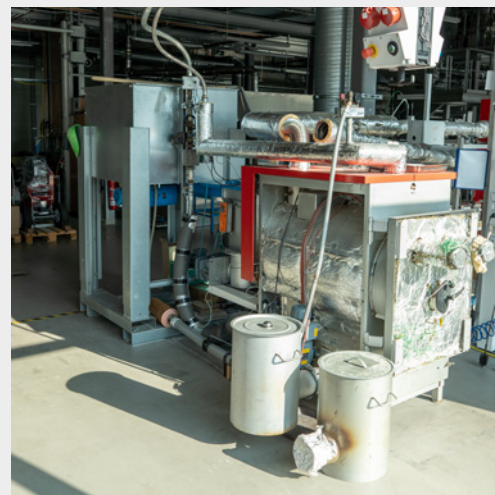
Fig. 18: Test beds for biogas digestion tests, biomass gasification tests and combustion trials
