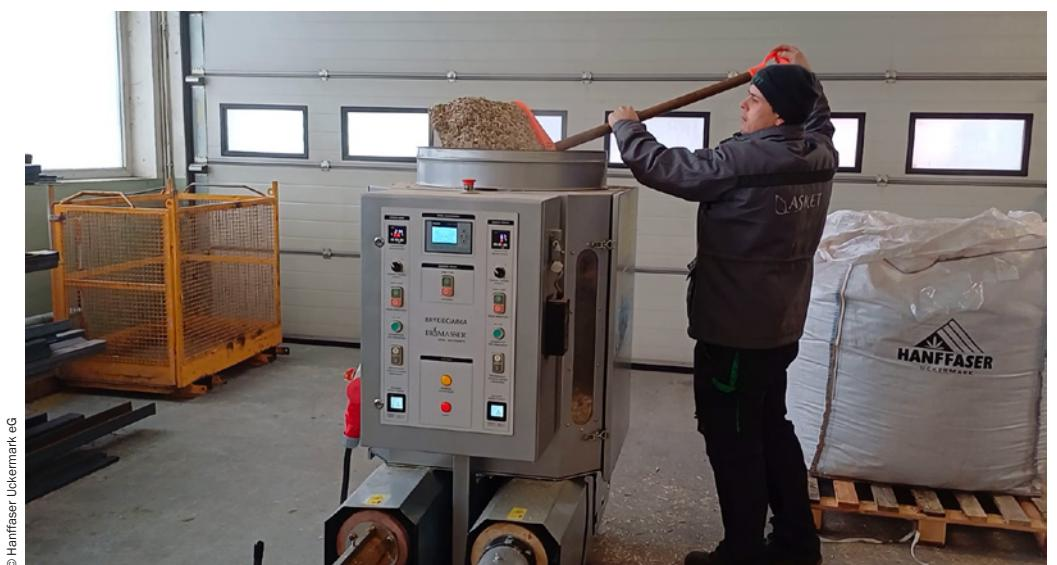
**Fig. 53:** Pressing hemp briquettes using a thermal process
