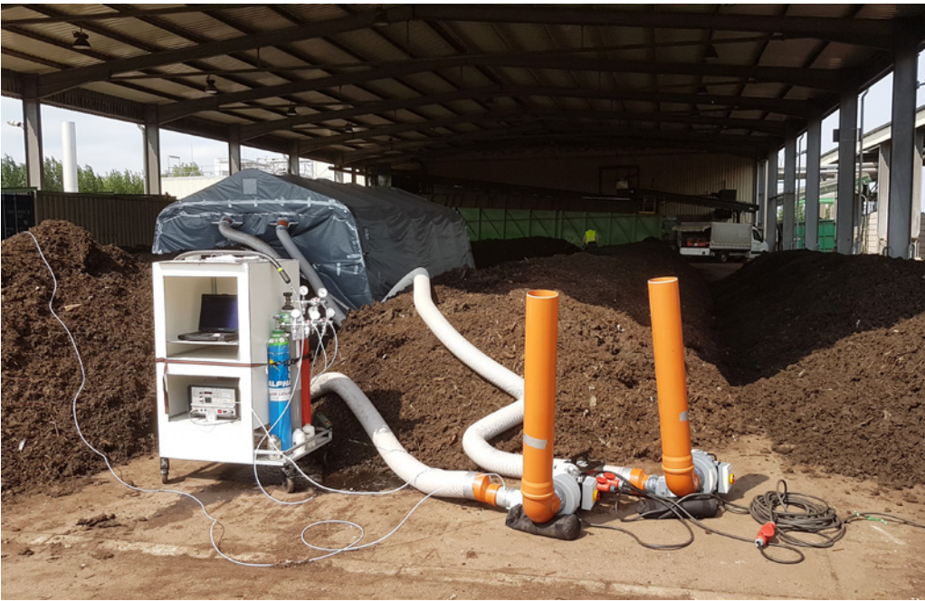
Fig. 23: Test setup of the wind tunnel measurements with use of the FID on the rotting of fermentation plant A04 in June 2019
