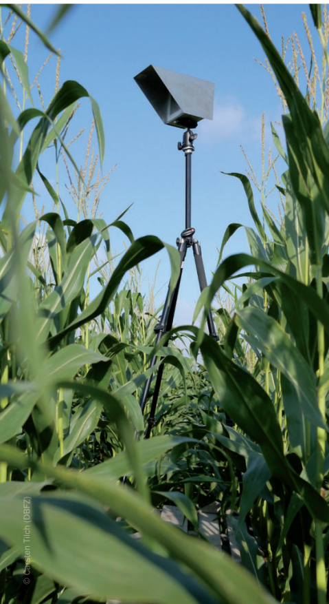
Figure 20: Reflector module of a laser spectrometer to measure methane concentration around biogas plants
