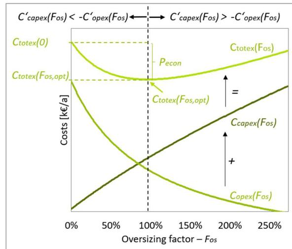
Figure 4.5: Graphical demonstration of parameters to determine the economic DSM potential.
