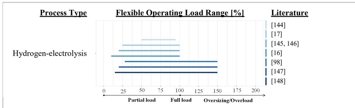
Figure 2.7: Flexible operating load range of hydrogen electrolysis as found in literature.
