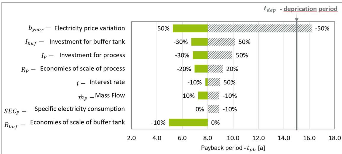
Figure 4.10: Tornado graph for the sensitivity analysis of all relevant factors affecting the payback period of DSM implementation.
