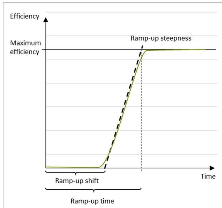
Figure 5.5: Exemplary graphical demonstration of ramping behavior of unit operation.
