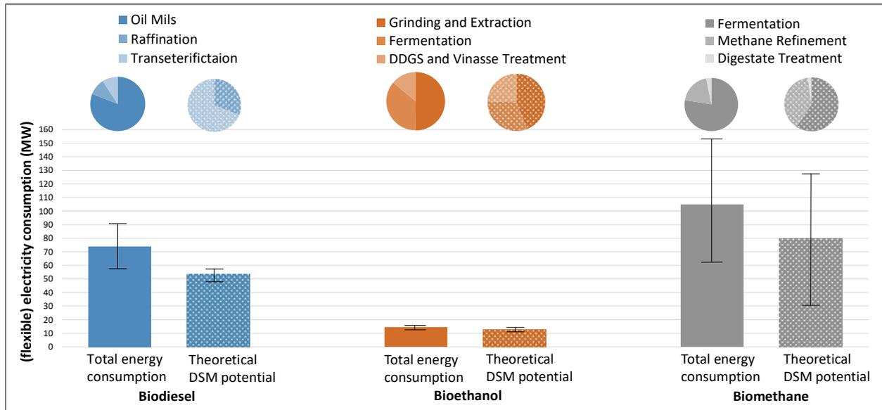
Figure 3.4: Total electricity consumption and theoretical DSM potential of Biodiesel, Bioethanol, and Biomethane in Germany for the year 2019.
