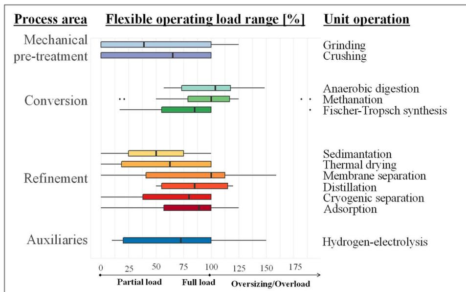
Figure 2.8: Distribution of the operating load range per unit operation found in this review.
