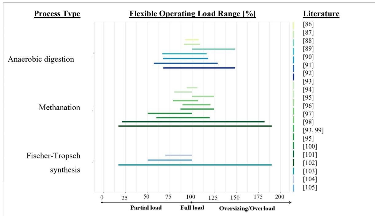
Figure 2.5: Flexible operating load range of conversion processes as found in literature.
