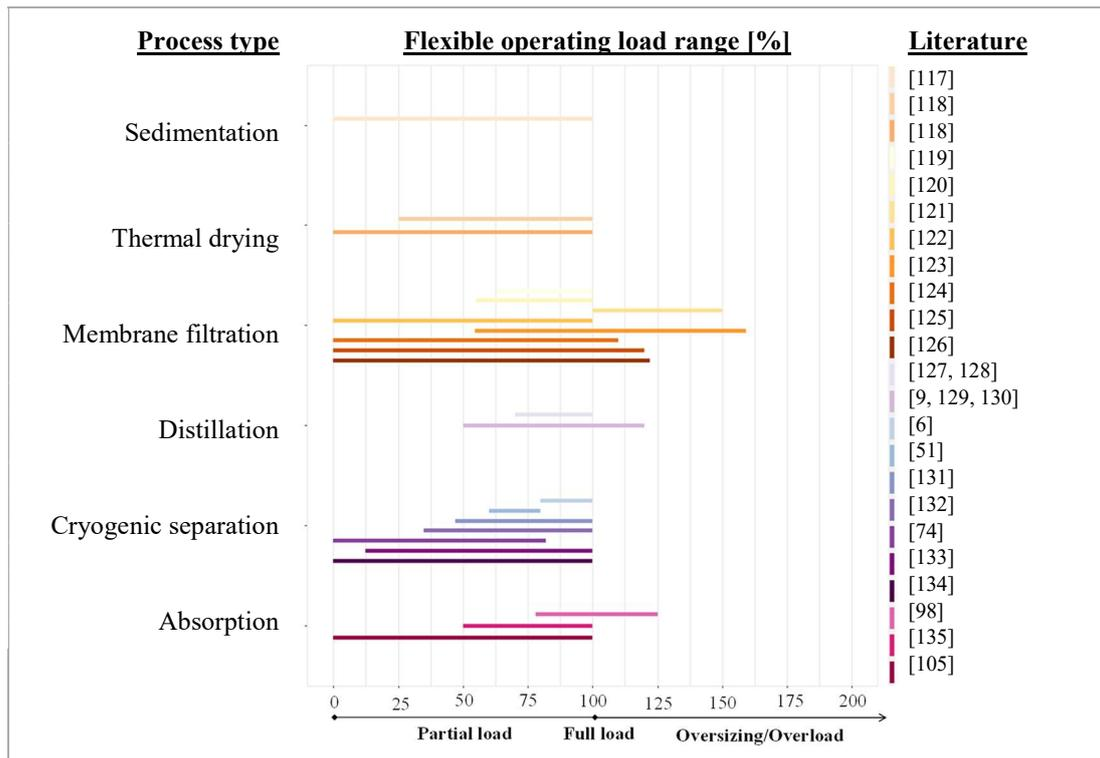
Figure 2.6: Flexible operating load range of solid, liquid, and gas refinement as found in literature.
