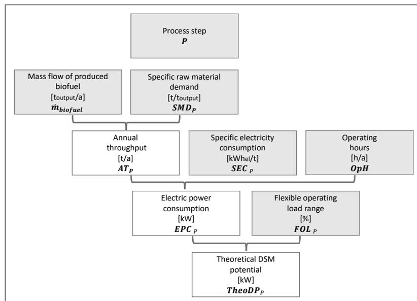
Figure 3.1: Method for calculating the theoretical DSM potential of process steps.
