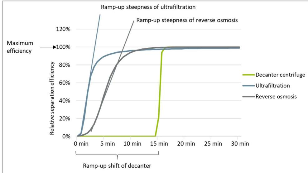
Figure 5.8: Ramp-up behaviour of digestate separation processes regarding their separation efficiencies as implemented in the dynamic simulation.
