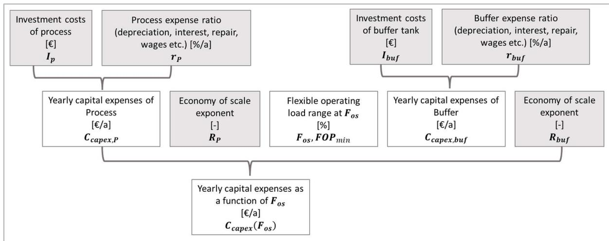
Figure 4.4: Method to calculate the most important parameters to determine the capital expenditure as a function of oversizing.
