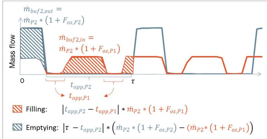
Figure 5.4: Graphical demonstration of the development of equations for buffer tank volumes dependent on the oversizing of up- and downstream processes.
