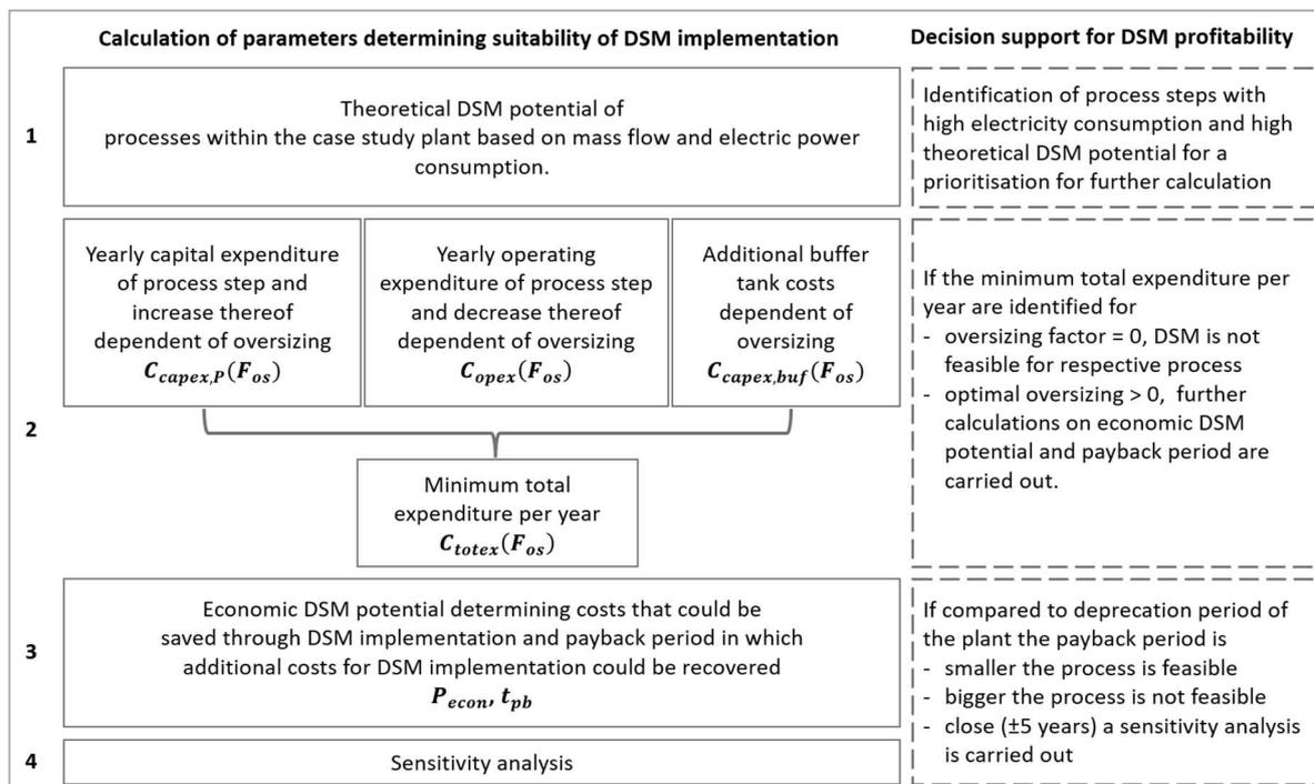
Figure 4.1: Decision support tool to evaluate essential economic parameters for the decision of a DSM implementation for continuously operated processes.
