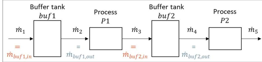
Figure 5.3: Exemplary block flow diagram of process cascade with intermediate buffer tanks.
