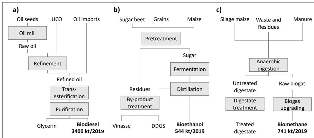
Figure 3.2: Reference concepts for biofuel production a) Biodiesel b) Bioethanol c) Biomethane.
