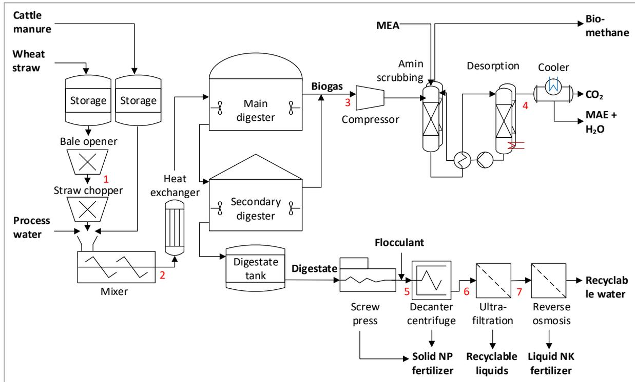
Figure 4.6: Simplified scheme of the biorefinery concept used as a case study, with necessary buffer tank locations indicated in red.
