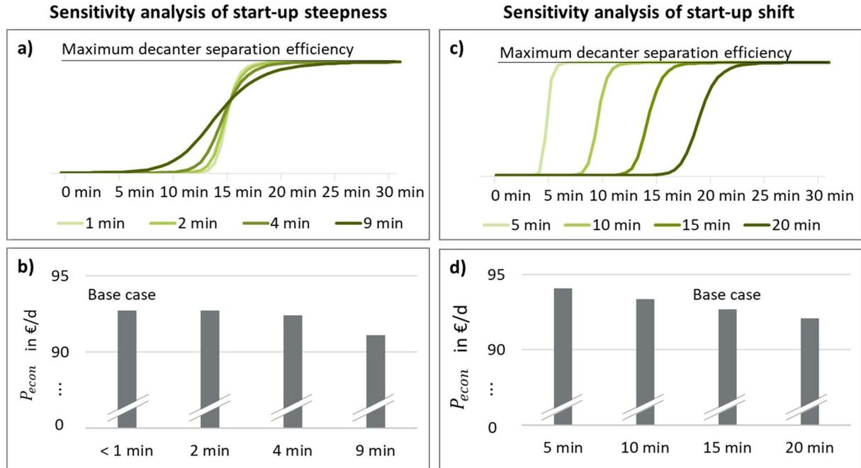
Figure 5.12: Results of sensitivity analysis of ramp-up behaviour of decanter centrifuge.
