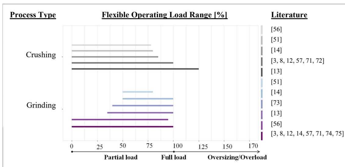
Figure 2.4: Flexible operating load range of mechanical pre-treatment processes as found in literature.
