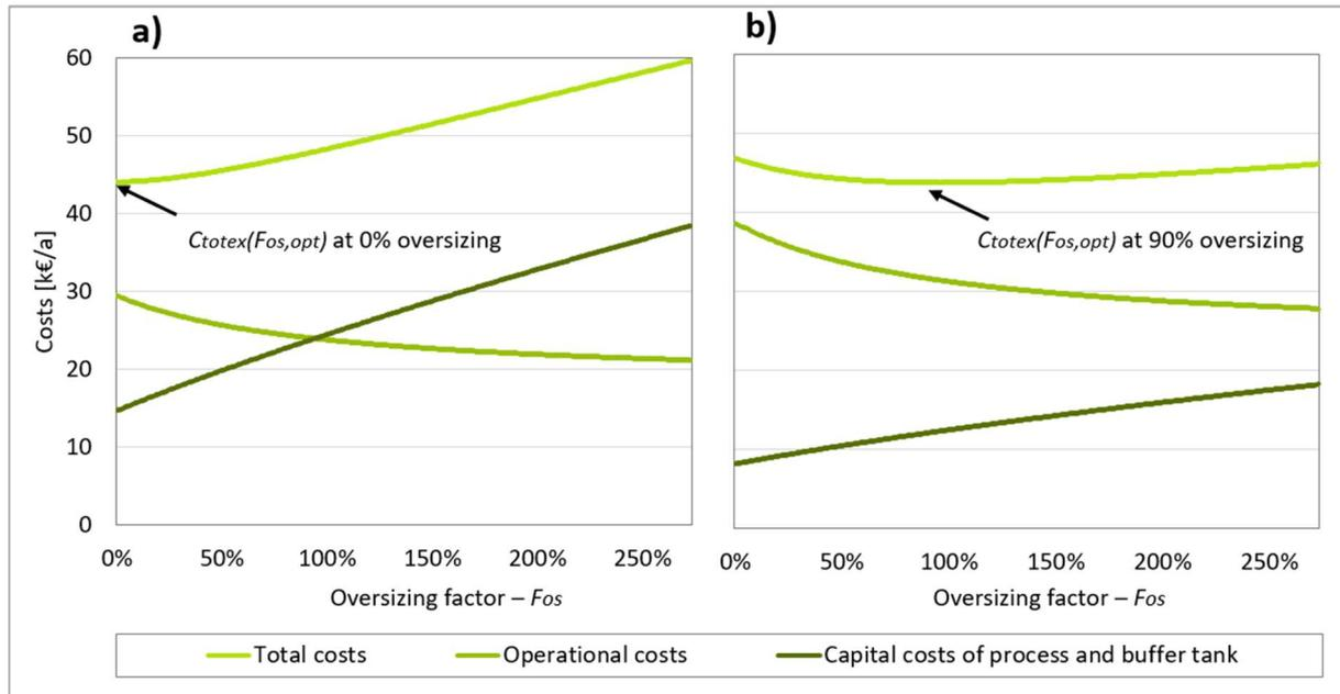
Figure 4.8: Exemplary demonstration of operational, capital, and total expenditure as a function of oversizing of a) screw press separator and b) bale opener.
