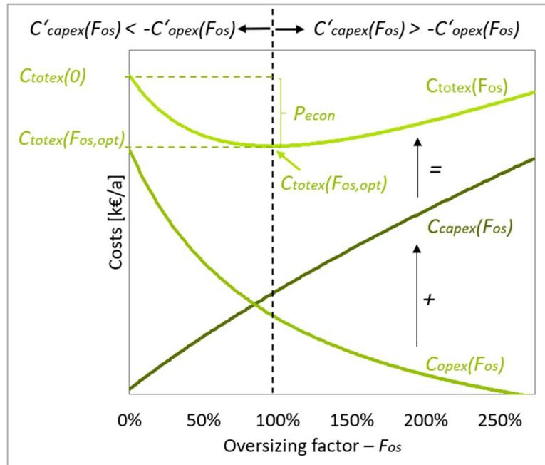
Figure 5.1: Graphical demonstration of parameters to determine the economic DSM potential. [228]
