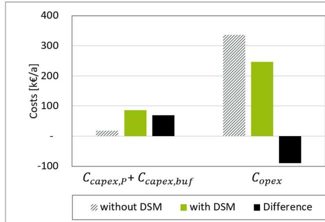
Figure 4.9: Cost structure of the demand side management impact for the decanter centrifuge.
