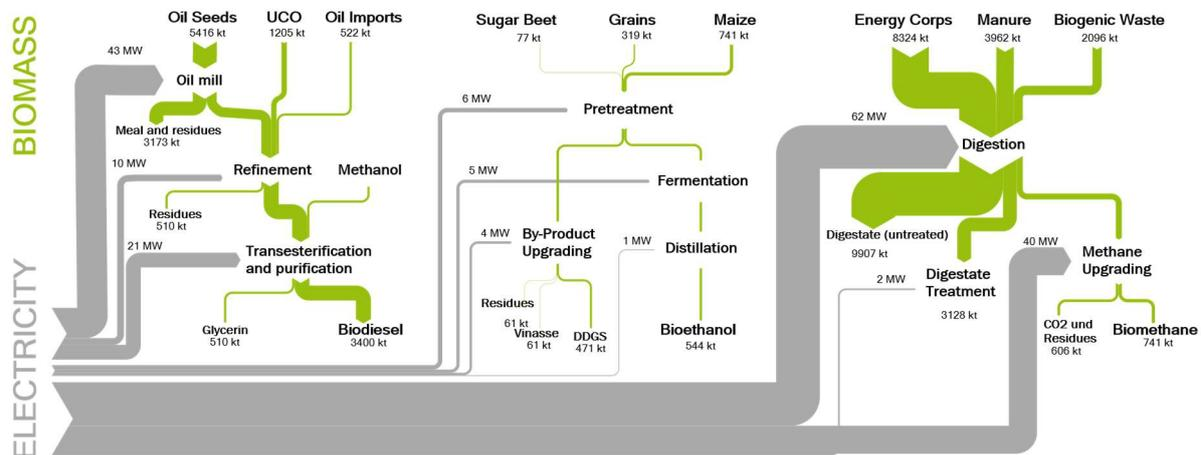
Figure 3.3: Material flows for biofuel production in Germany for a) Biodiesel, b) Bioethanol c) Biomethane.
