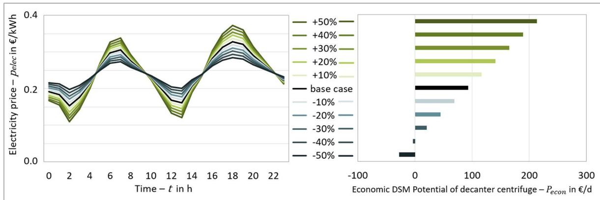
Figure 5.14: Sensitivity analysis of influence of intensity of electricity price fluctuations on economic DSM potential of decanter centrifuge.
