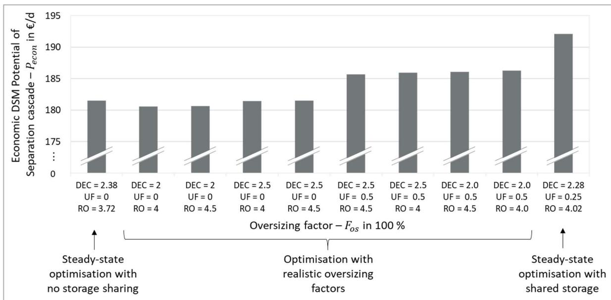
Figure 5.9: Steady-state optimization results of digestate separation cascade at ideal and realistic oversizing factors for decanter centrifuge (DEC), ultrafiltration (UF), and reverse osmosis (RO).
