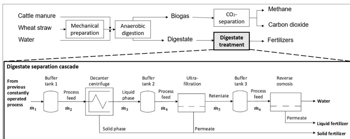
Figure 5.7: Digestate separation cascade of the biomethane biorefinery for which demand side management implementation was investigated (as described in [216]).
