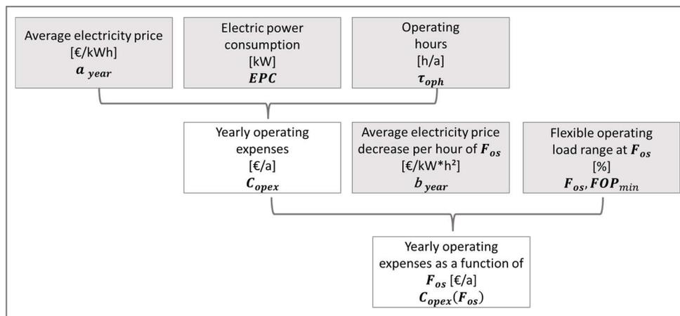
Figure 4.2: Method to calculate the most important parameters to determine operating expenditure as a function of oversizing.
