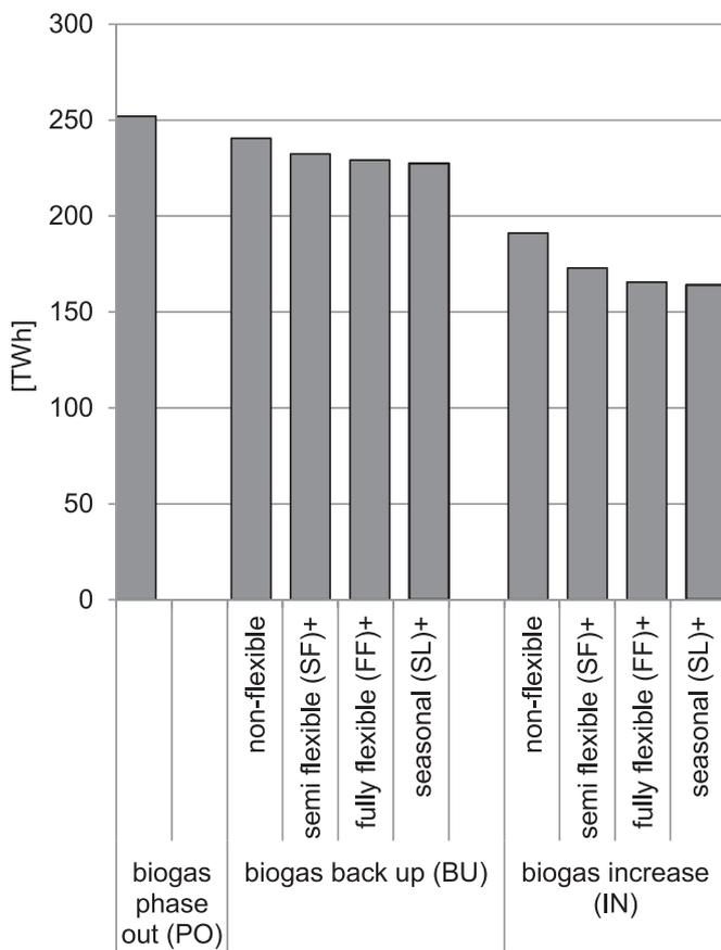
Fig. 6. Surplus generation in all scenarios with regard to flexible power generation in existing plants (+) and in the period of 2016–2035. In addition, results of non-flexible power generation in extension paths *biogas back up* and *biogas increase* are shown.
