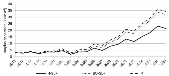
**Fig. 5.** Surplus generation in the *biogas increase* and *biogas back up* extension paths with seasonal mode of operation and flexible existing biogas plants (IN-SL+ | BU-SL+) as well as in the reference scenario (R) for the period of 2016–2035.
