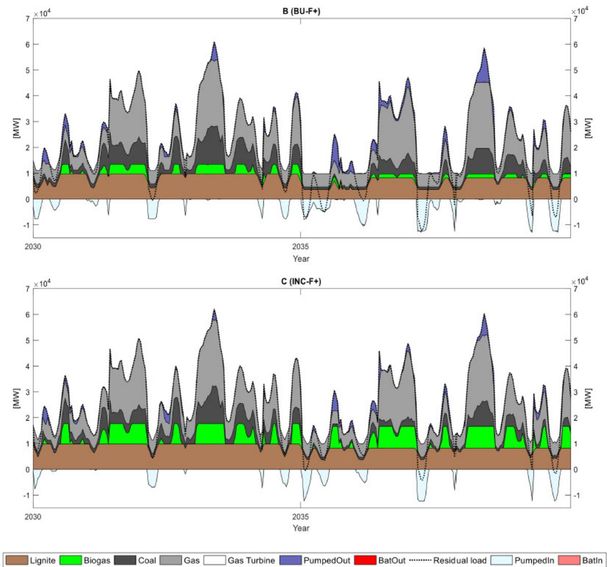
**Figure 3.** Residual load, biogas, and conventional electricity generation, as well as the operation of the storage technologies in the years 2030 and 2035 in the scenarios REF (A); BU-F+ (B) and INC-F+ (C). PumpedOut: discharged electricity from pumped-storage plants. BatOut: discharged electricity from Li-ion batteries. PumpedIn: charged electricity in pumped-storage plants. BatIn: charged electricity in Li-ion batteries.
