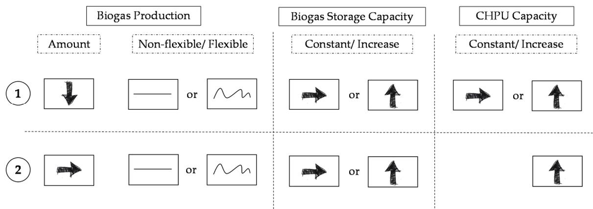
Figure 1: Overview of flexibilization approaches of existing biogas plants. No. 1: Flexible power generation when biogas production is reduced. No. 2: Flexible power generation when biogas production is set as constant.
