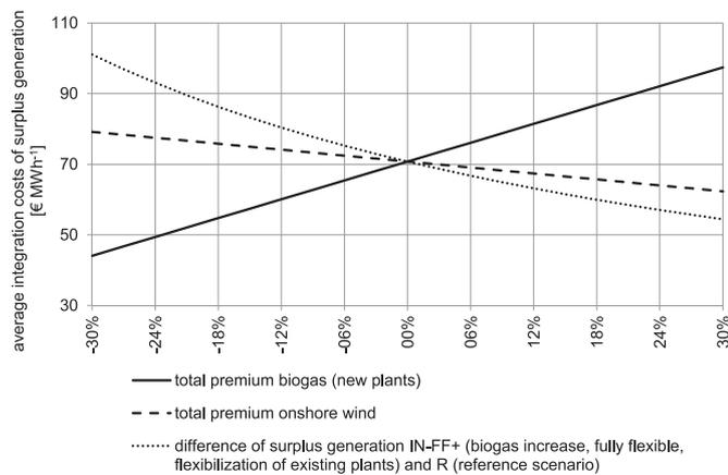
**Fig. 9.** Sensitivity analysis of the *biogas increase* extension path, fully flexible mode of operation and flexible power generation from existing biogas plants (scenario IN-FF+) for the period of 201–2035.
