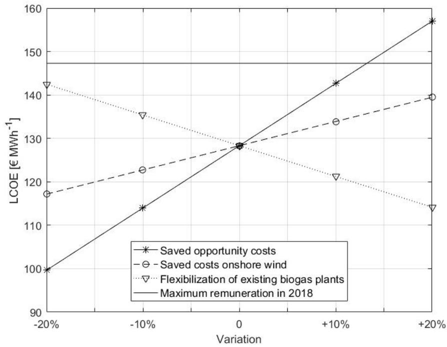
Figure 7: Maximum LCOE of new biogas installations that allows operations to be economically feasible in the scenario BU-F+ and an early phasing-out of lignite- and coal-fired power plants. The commissioning year is 2018.
