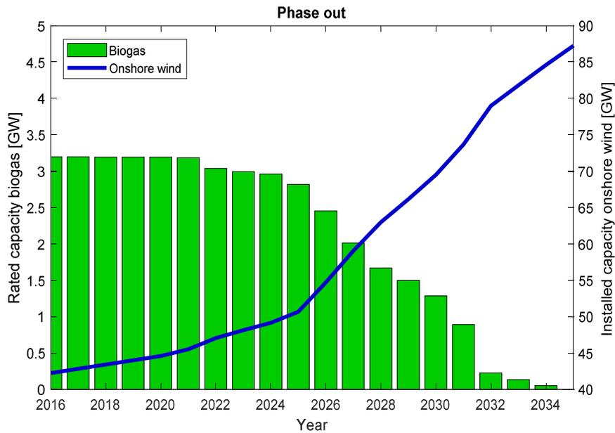
Figure 3: Installed capacities of onshore wind and rated capacities of biogas plants in the biogas extension path *phase out* (adapted from Lauer and Thrän [2018]).
