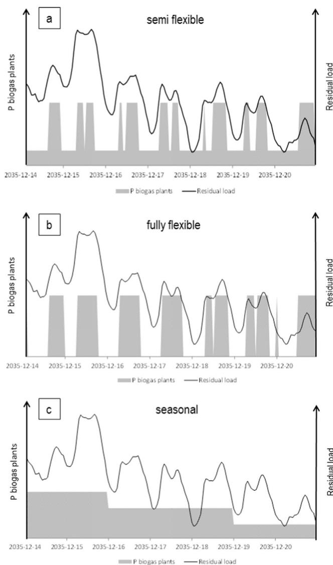
**Fig. 3.** Overview of modes of operation used in this paper (a: semi flexible, b: fully flexible and c: seasonal). The example shown here is electricity generation from biogas plants in the biogas increase extension path based on residual load within seven days in 2035. Abbreviation: P = power.
