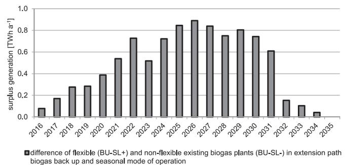
Fig. 8. Temporal distribution of additional surplus generation by non-flexible (BU-SL-) compared to flexible power generation in existing biogas plants (BU-SL+) in the *biogas back up* extension path and seasonal mode of operation.
