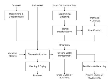
Figure 28 - Flow chart of biodiesel production process (Hamilton 2004)
