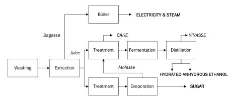
Figure 10 - Simplified overview of the industrial sugar and ethanol production process (Smeets et al. 2006)
