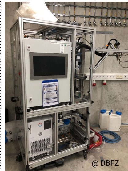
Upscaling HRD system in Hydrothermal membrane system (HTMV) for integration to 10 L reactor
