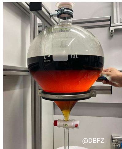
View into the modified HTMV (left) and phase separation of the organic phase (right) (© Andrés C. Acosta, 2026).
