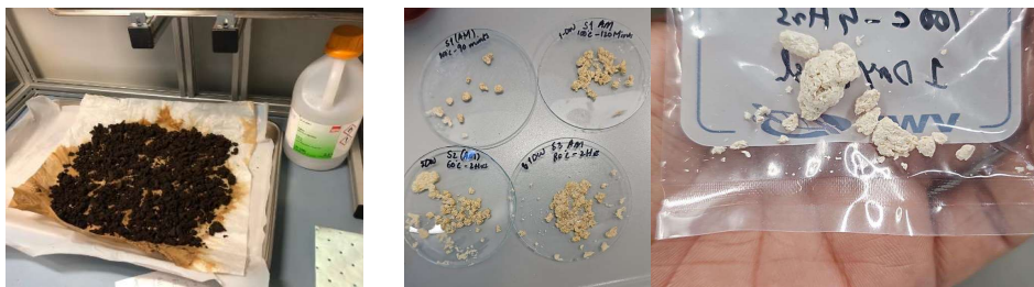
Pulp obtained after fractionation (left) and acidic bleached pulp (right) @ DBFZ
