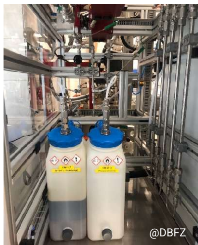
View into the modified HTMV (left) and phase separation of the organic phase (right) (© Andrés C. Acosta, 2026).
