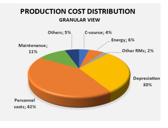
Figure 3 - Cost composition for baseline process conditions
