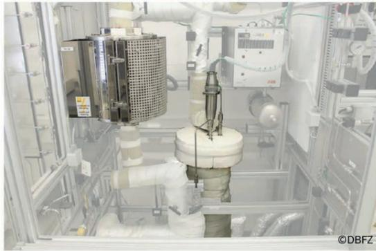
Left: Adiabatic tube reactor (electrically heated,  $T_{\max} = 600\text{ °C}$ )
