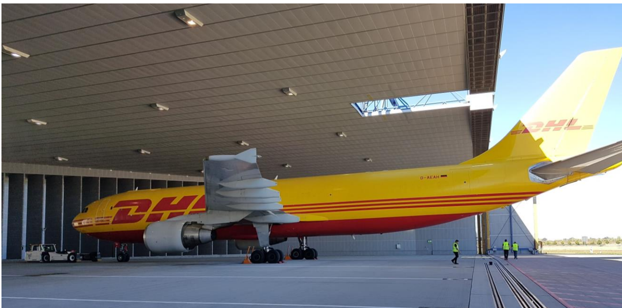
Fig. 5 The A300-600 for ground measurement in the engine test run facility
