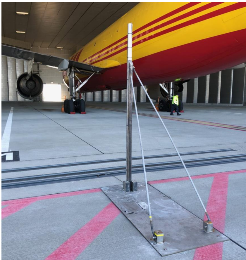
Fig. 6 Sampling probe in position in the engine test run facility
