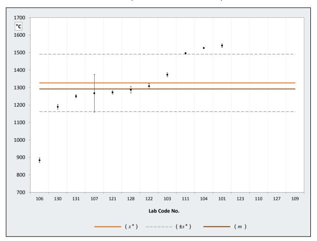
Deformation temperature - DT - Torrefield pellets
