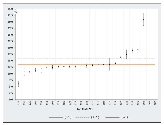
loss of mechanical durability -  $D_{U \, \text{loss}}$  - Torrefield pellets
