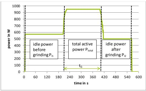
Figure 1: Typical curve of the power measurement including the three sections
