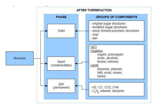
Figure 1: Products formed during torrefaction of biomass (source: Bergmann 2005)
