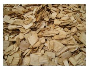
Figure 4: Feedstock suitable for ECN torrefaction
