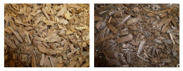
Figure 13: Beech wood treated in CENER pilot plant (left original sample, right torrefied sample)
