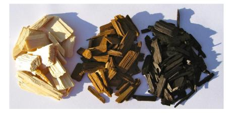
Figure 8: Torrefied wood chips
