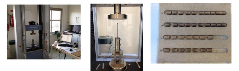
Determination of: Compression energy, friction and quality analysis of pellets
