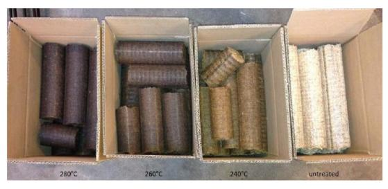
Material torrefied at ECN: Spruce and Bamboo Briquetting tests DTI in cooperation with CF Nielsen
