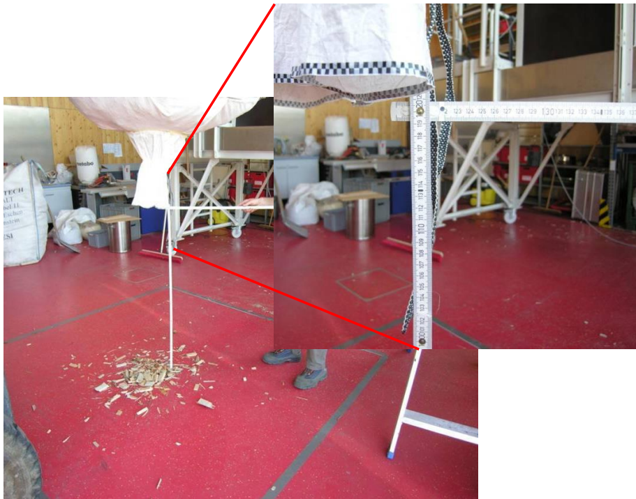
Figure 27: Position of the filled big bag before opening the lower outlet for unloading
