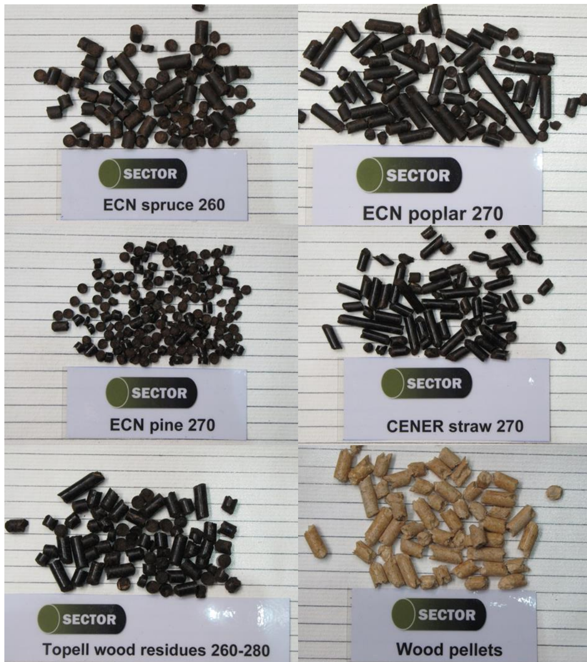
Figure 33: The pellet grades used in the experiments at VTT. Distance between the lines in photos was 10 mm.
