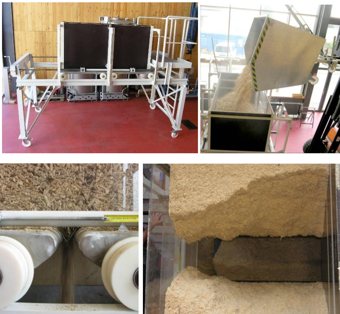
Figure 25: Apparatus for bridging tests: Top left: complete box with opening floor driven by crank handle. Top right: filling of the box with sample material. Bottom left: beginning of floor opening with measuring rule showing the dimension of gap while material starts to fall through. Bottom right: fully collapsed bridge (view from top)
