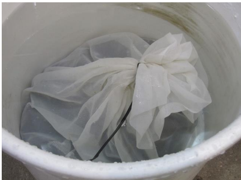
Figure 34: A pellet sample submerged to water in a filtration bag during the water immersion test.
