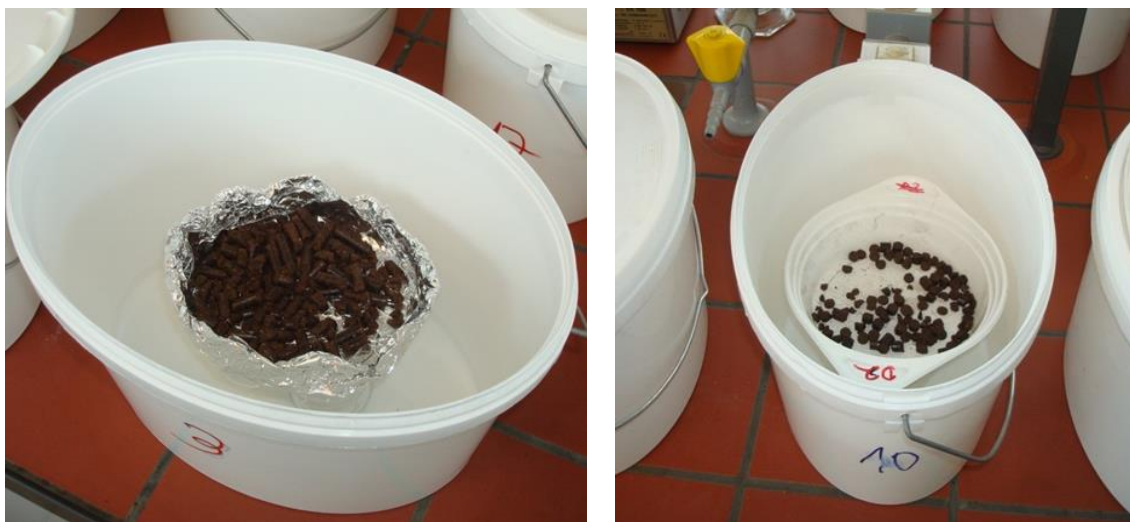
Figure 1: Experimental setup for NaCl (right) / K 2 SO 4 (left) exposure tests
