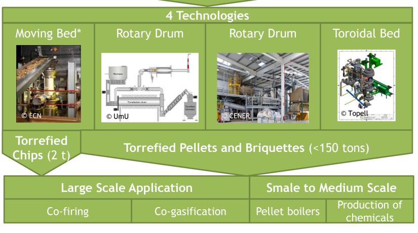
\* And the resulting Andritz/ECN technology, successfully demonstrated in Denmark at a scale of 1 ton/h
