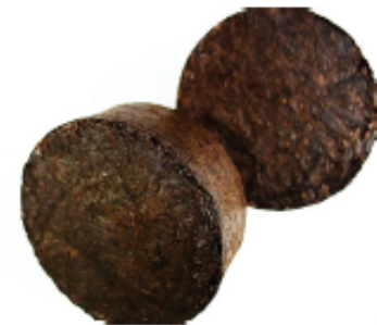
Test briquettes from ACB material source: TU-Freiberg
