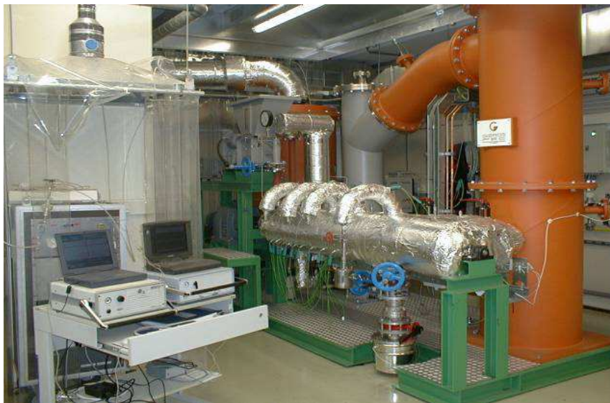
5 kg/h Auger reactor (screw reactor)
