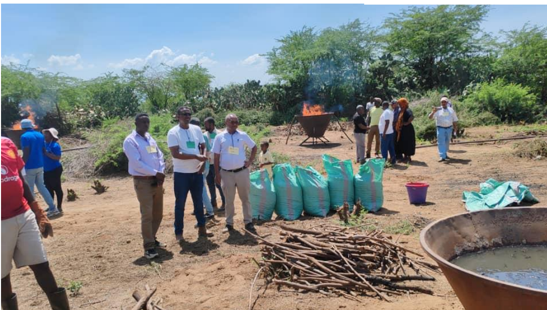
Bottom: Burning Kon-Tiki in the background; Prosopis juliflora biomass, biochar in bags, tools (buckets and plane) and a water quenched Kon-Tiki in the foreground, beside the Ethiopian study tour participants.
