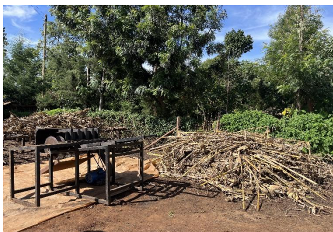
Semi automatic maize straw cutting machine.
