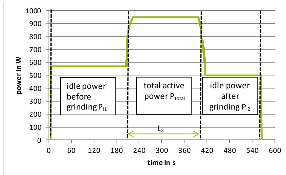
Figure 1: Typical curve of the power measurement including the three sections
