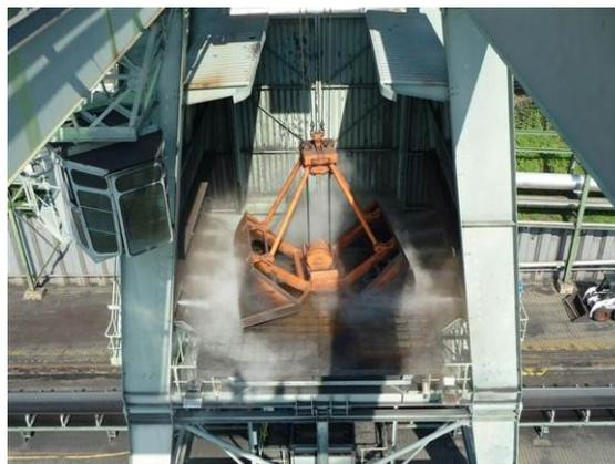
**Figure 22: Un-loading with water dispersion system in operation during full scale test at RW**
