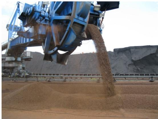
**Figure 25: Reclaimer in operation handling thermally treated biomass pellets during full scale test at RW**
