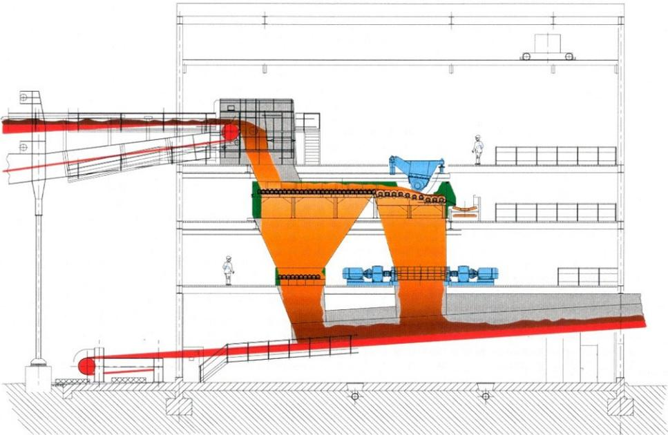
Figure 8: Combined crushing and screening unit
