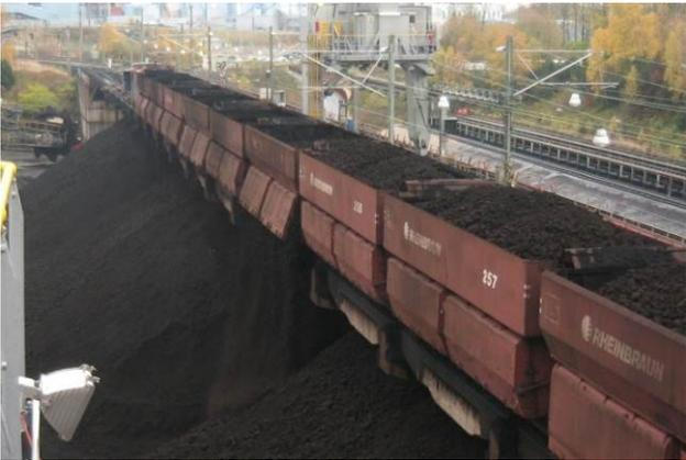
Figure 7: Train unloading into ditch bunker
