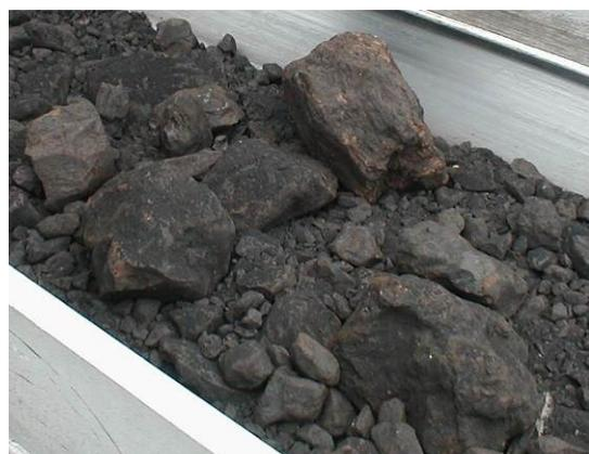
**Figure 5: Raw lignite on conveyor belt**
