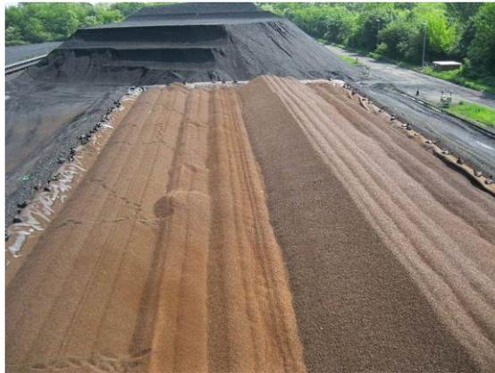
**Figure 24: A pile of thermally treated biomass pellets from top of reclaimer during full scale test at RW**
