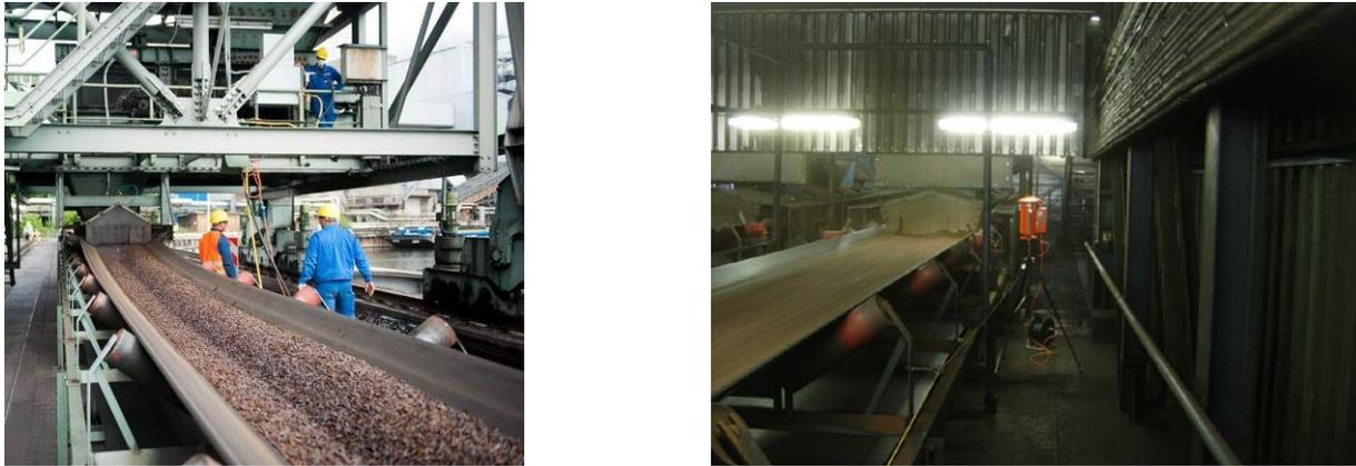
**Figure 23: From harbour hopper to conveyor belt with water dispersion system (left) and at transition station (right) during full scale test at RW**
