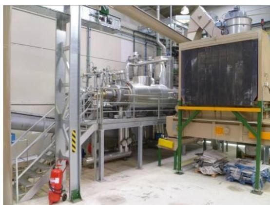
Figure 11: Torrefaction unit in CENER facilities
