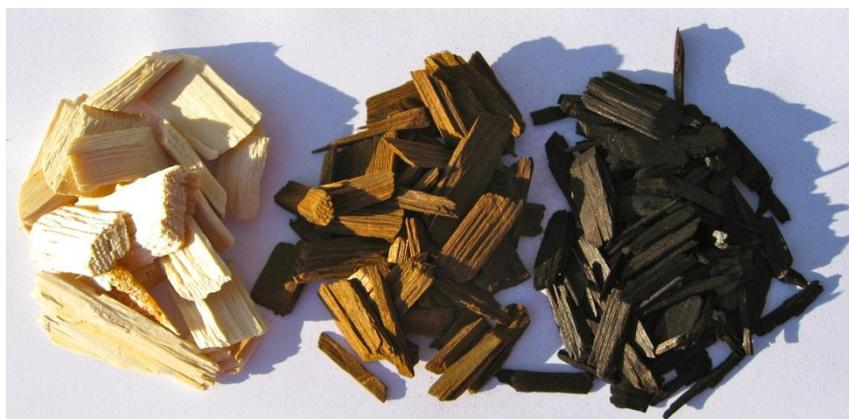
Figure 8: Torrefied wood chips
