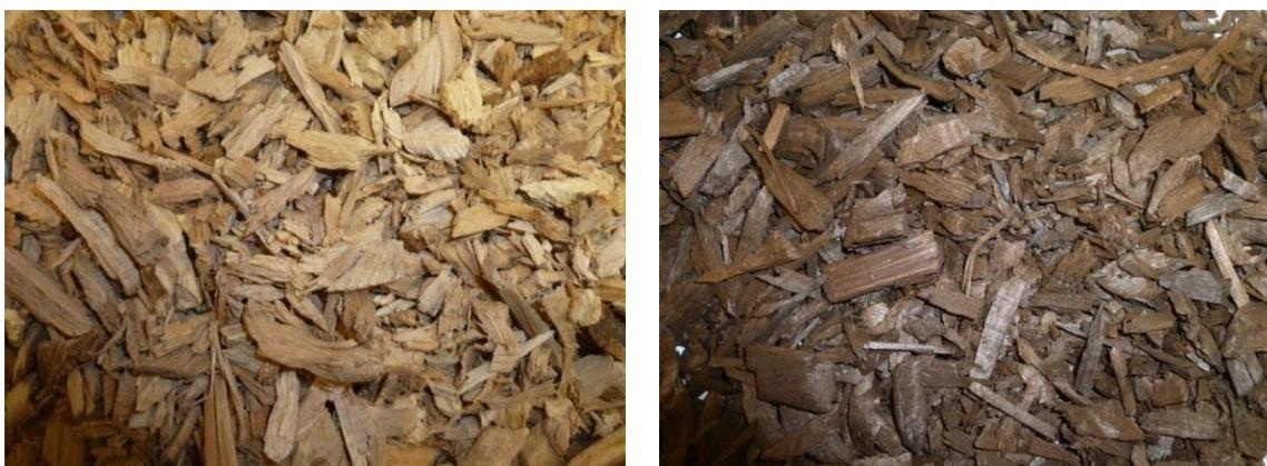
Figure 13: Beech wood treated in CENER pilot plant (left original sample, right torrefied sample)
