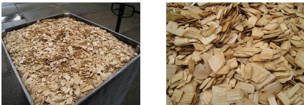
**Figure 4: Feedstock suitable for ECN torrefaction**
