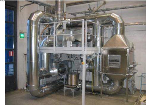
Climatic testing chamber for determination of equilibrium moisture content
