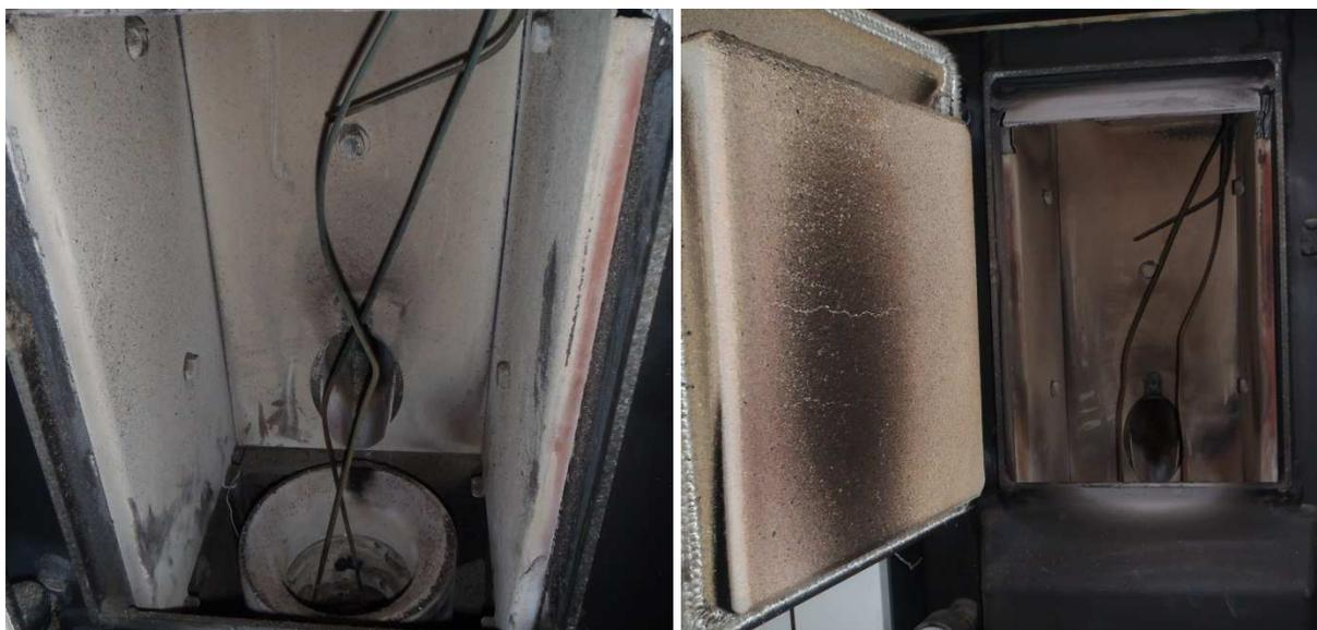
**Figure 37: Combustion chamber of boiler4 before(left) and after (right) the operation with spruce\_260.**
