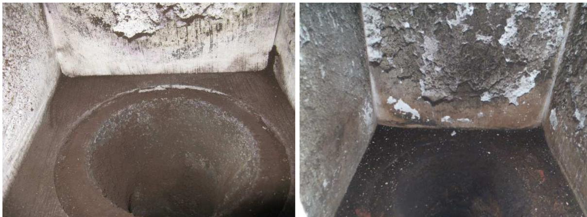
**Figure 36: Combustion chamber of boiler1 after the operation with spruce\_raw (left) and spruce\_260 (right).**
