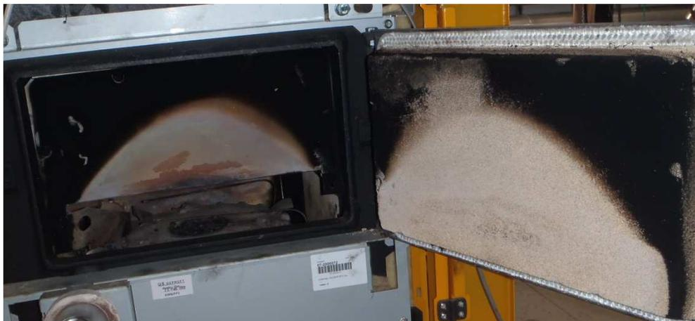
**Figure 35: Soot-covered surfaces inside the combustion appliance (Boiler2)**
