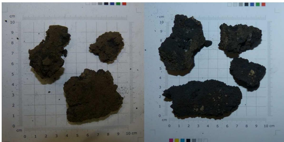
Figure 23: Agglomerated ash particles from the bottom ash (left picture) and grate ash (right picture) from Boiler 1
