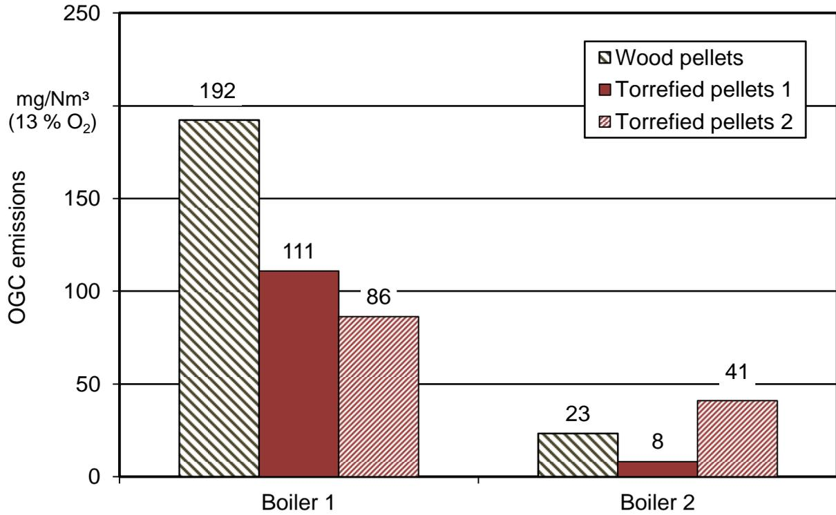
Figure 16: OGC emissions at variable load according to standard load cycle
