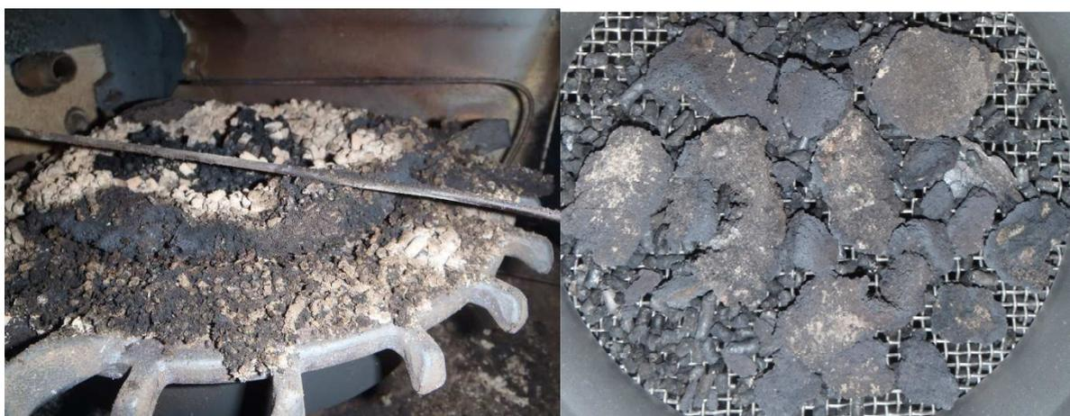
**Figure 18: Agglomerations of spruce\_260 on the grate of Boiler2 (left) and after sieving process (right).**
