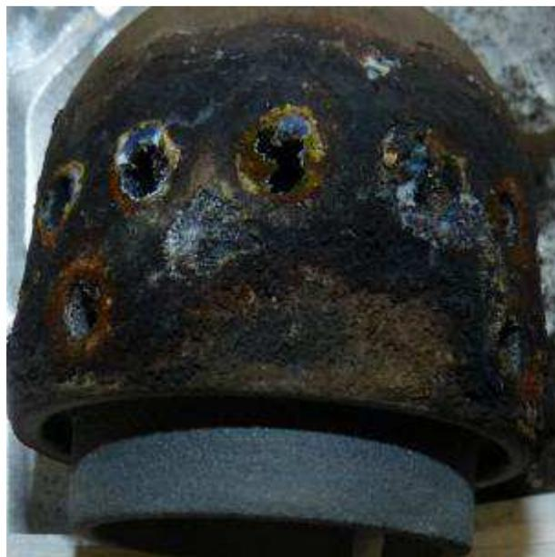
**Figure 25: Slag formation and clogging of air inlets on the hemispherical primary air head of Boiler 2 after long-term test using Torrefied pellets 1. Molten ash is beginning to block the nozzles for primary air supply.**
