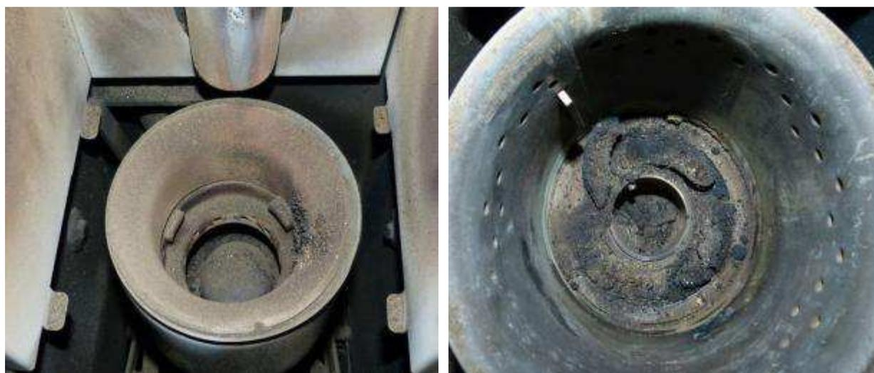
**Figure 24: Slag formation and deposits in Boiler 2 after long-term test with Torrefied pellets 1. In the picture right the hemispherical primary air head is removed. This head is show in Figure 25.**
