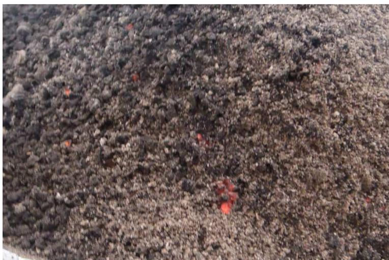
**Figure 17: Glowing particles in bottom ash of Boiler4, test fuel spruce\_260.**
