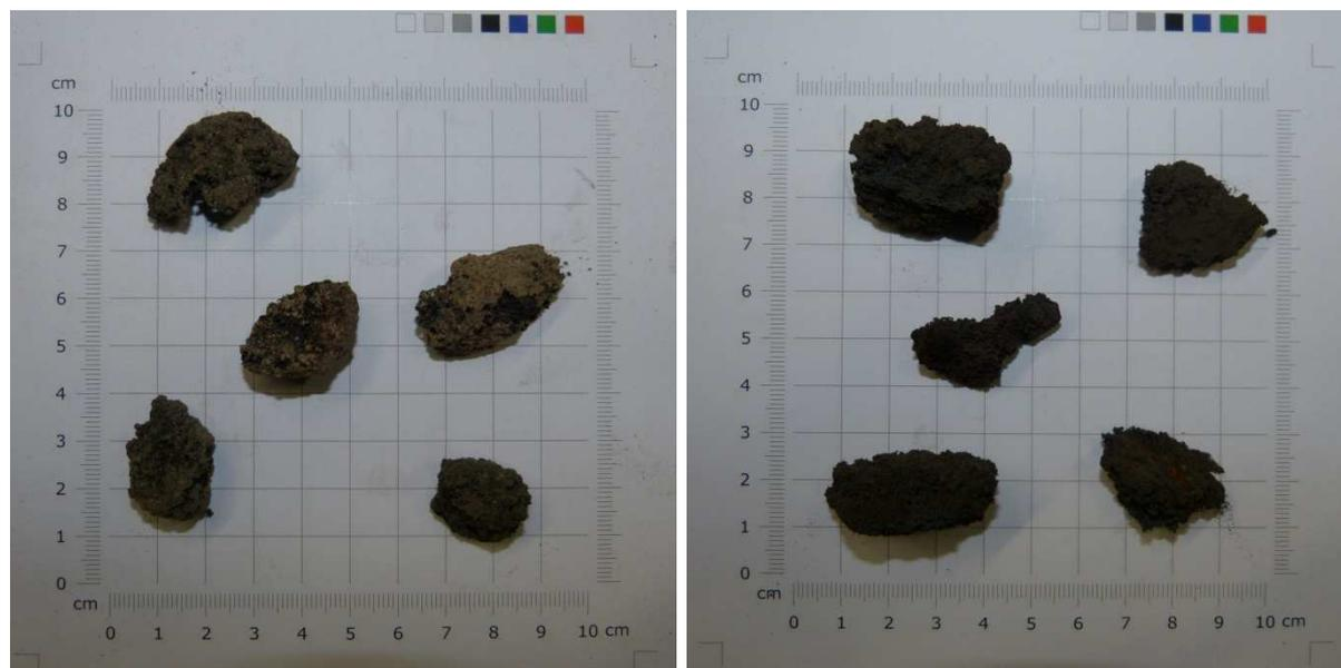
**Figure 26: Agglomerated ash particles from the bottom ash (left picture) and grate ash (right picture) from Boiler 2**
