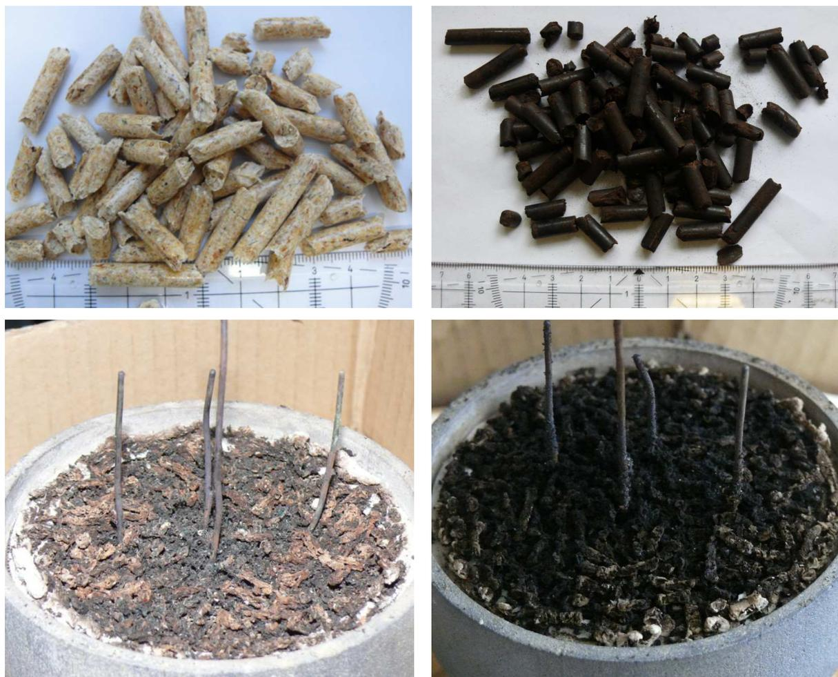
**Figure 18:** Photos of the fuel before (above) and the ashes (below) after the test run
