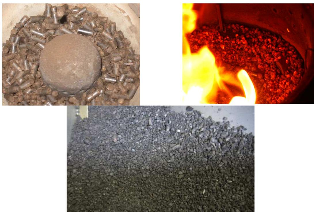
**Figure 20:** Pictures of the burner and the grate ash during test runs with TOPELL\_spruce (furnace settings 1)
