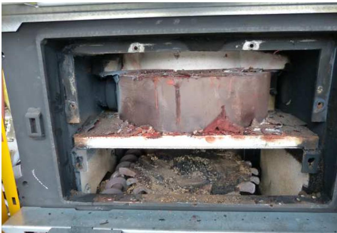
Figure 22: Slag formation and deposits in Boiler 1 after long-term test (Torrefied pellets 1)
