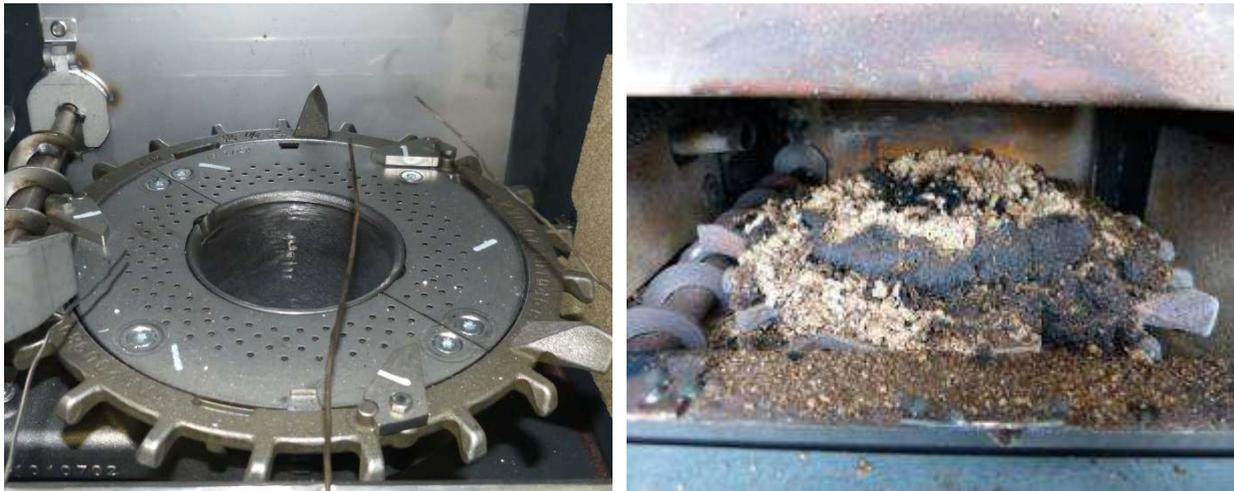
**Figure 21: Slag formation in burner unit of Boiler 1 after long-term test (Torrefied pellets 1). Left picture: clean burner unit before the long-term test. Right picture: burner unit after the tests.**
