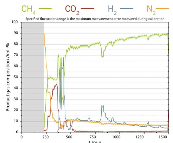
Fig. 5: Course of the product gas composition in the start-up process of the catalytic methanation of biogas
