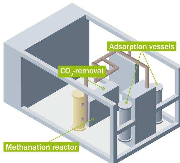
Fig. 1: Methanation module in the pilot plant with two adsorber vessels and a methanation reactor
