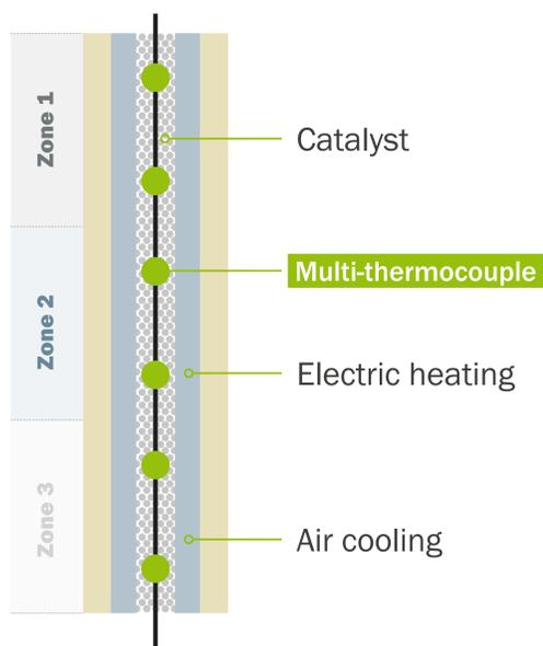
Fig. 2: Schematic structure of the methanation reactor
