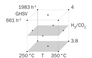
Fig. 5: Design of experiment for the catalyst evaluation
