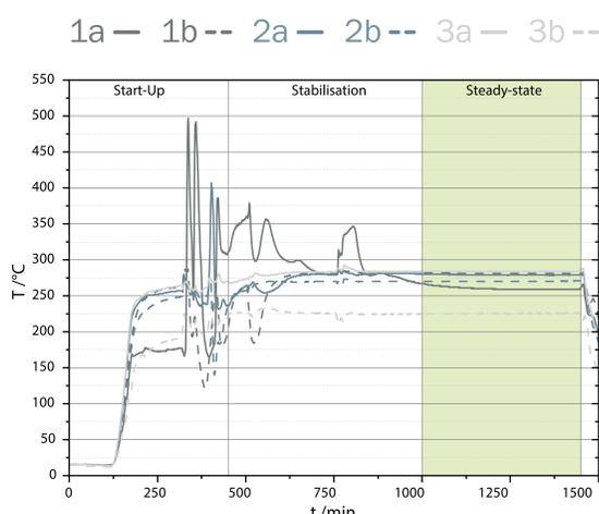
Fig. 4: Course of the reactor temperatures in the start-up process of the catalytic methanation of biogas
