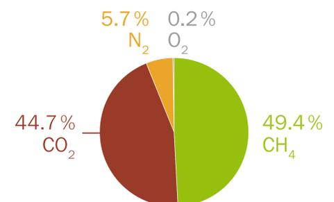
Fig. 3: Biogas composition in the storage tank at the start of the experiment
