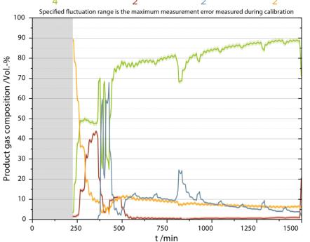
Nu2/Al<sub>2</sub>O<sub>3</sub>, T = 320 °C, p = 18 bar(g), H<sub>2</sub>:CO<sub>2</sub> = 4,  $\dot{V}_{biogas}$  = 60 L/h, GHSV = 449 h<sup>-1</sup>
