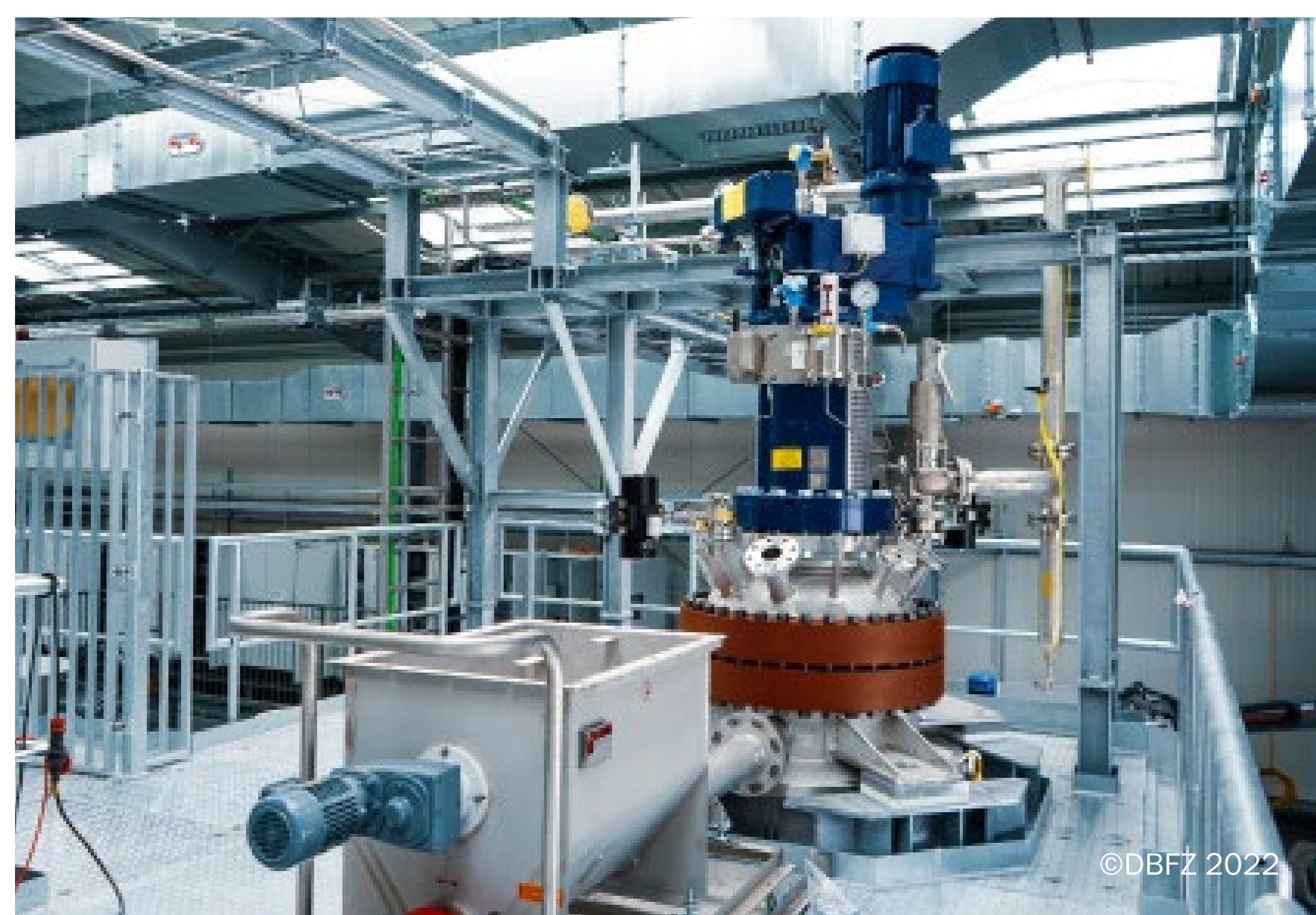
Fig. 3: Construction progress (anaerobic digestion line 2 with a plug flow reactor in the center of the photography)
