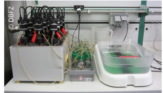
Batch-Test with AMPTS II-equipment by Bioprocesscontrol [DBFZ]
