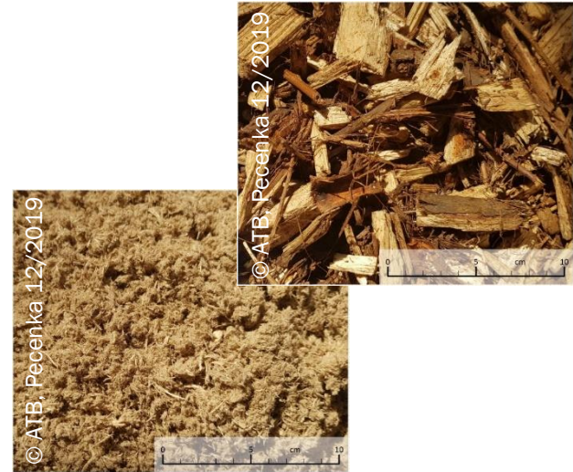
Poplar wood chips and fibres after extrusion [ATB, Pecenka 12/2019]
