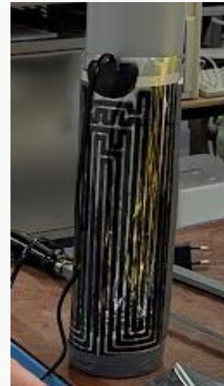
Fig 8: Heating pad, insulation, sample points and sensors
