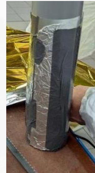
Fig 8: Heating pad, insulation, sample points and sensors
