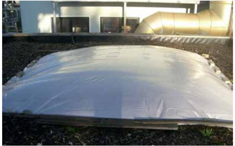
b) Measurement setup at an open biofilter [DBFZ]
