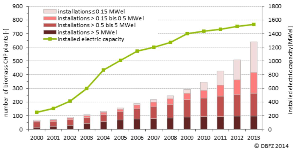
Figure 2-11: Development of solid biomass CHP plants in Germany from 2000 to 2013 (number of plants and installed electric capacity in MW<sub>el</sub>), without installations of the pulp and paper industry and small-scale CHP plants (< 10 kW<sub>el</sub>) (DBFZ, 2014)
