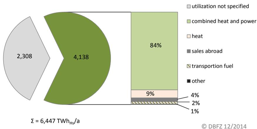
Figure 2-10: Biomethane utilization pathways in 2013 [TWh<sub>H<sub>2</sub></sub>] (own illustration based on the data of the German Energy Agency (dena) (Edel et al., 2014))
