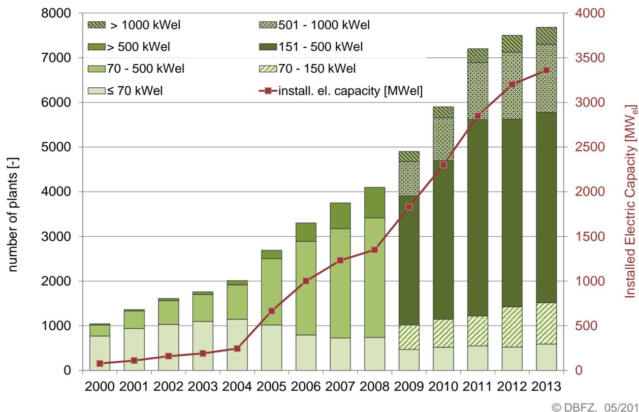
Figure 2-1: Development of biogas plants in Germany (number of plants and installed electric capacity in MW<sub>e</sub>) from 2000 to 2013, without biogas upgrading plants, landfill and sewage gas plants (DBFZ, 2014)
