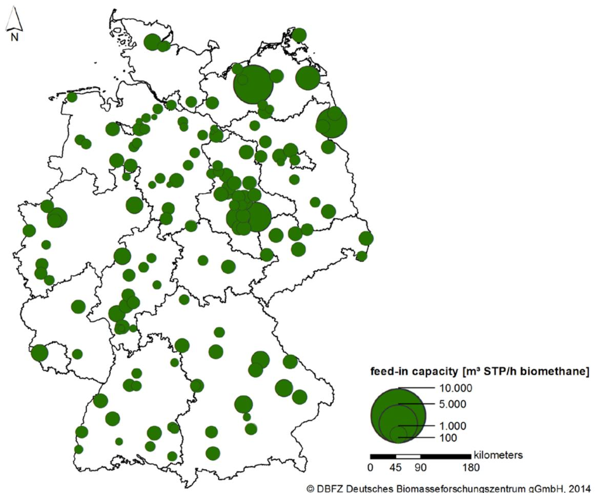
Figure 2-8: Distribution of biogas upgrading plants in Germany in 2013 (DBFZ, 2014)
