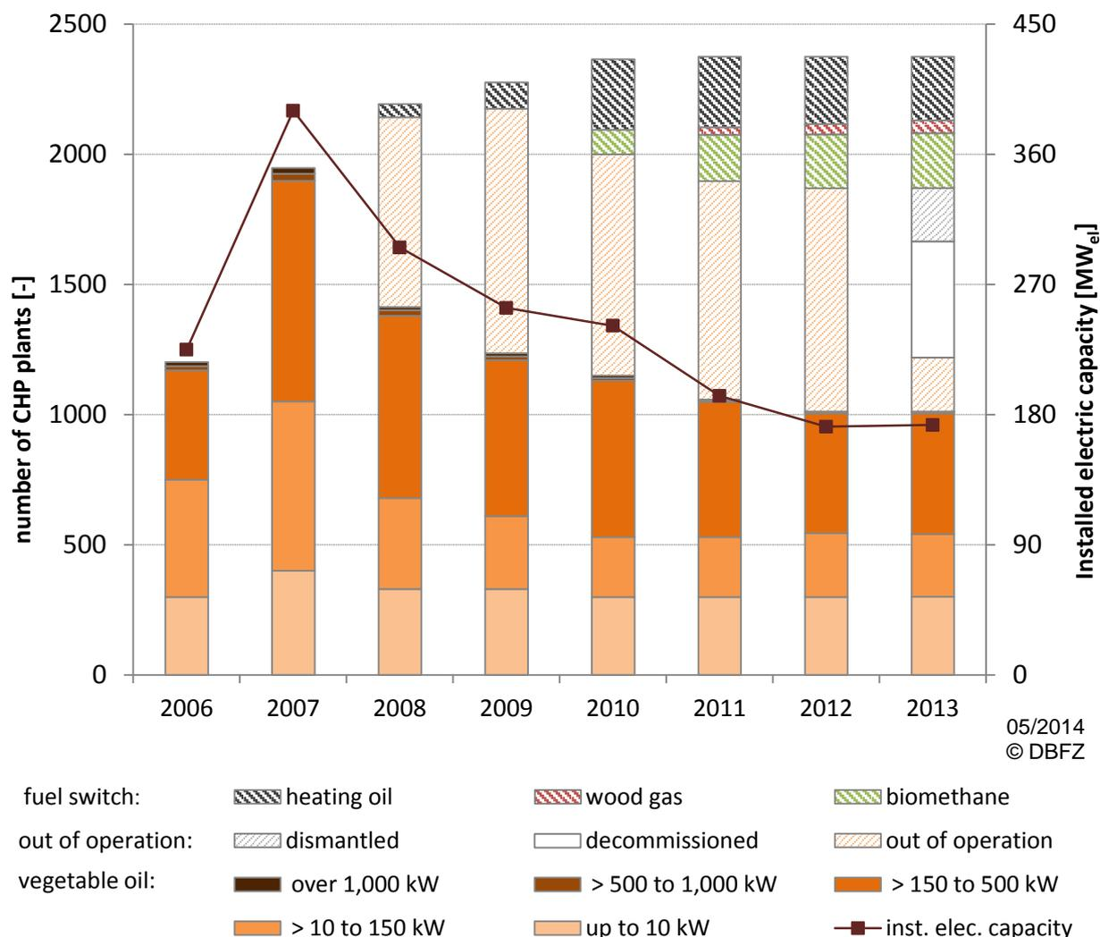
Figure 2-17: Development of vegetable oil CHP plants in Germany from 2006 to 2013 (number of plants and installed electric capacity in MW<sub>e</sub>) (DBFZ, 2014)
