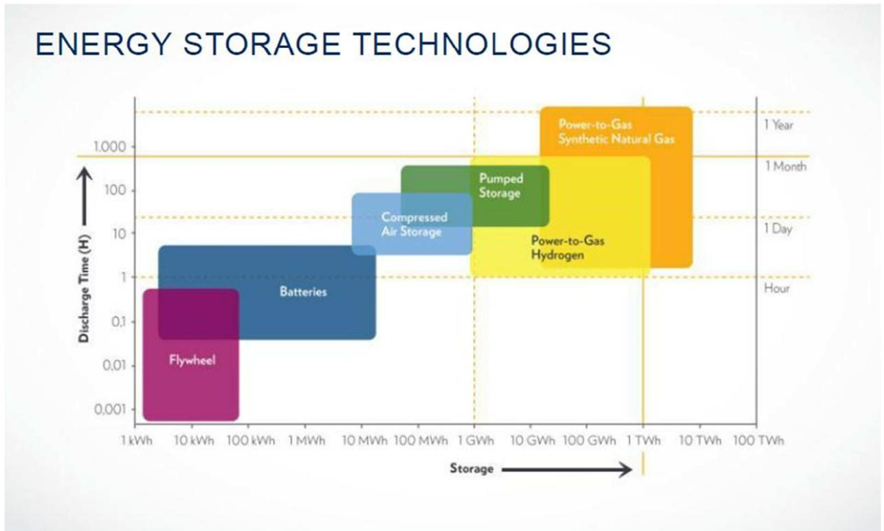
Figure 3-2. Energy storage technologies (Newton et al. 2013)
