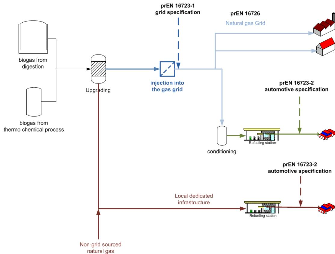
**Figure 2-4.** Schematic of the biomethane and natural gas transport system, showing in which points of the gas network the different standards of CEN/TC408 will apply; the point of entry for injection, and the point of use as automotive fuel. Source: CEN/TC408 working group.
