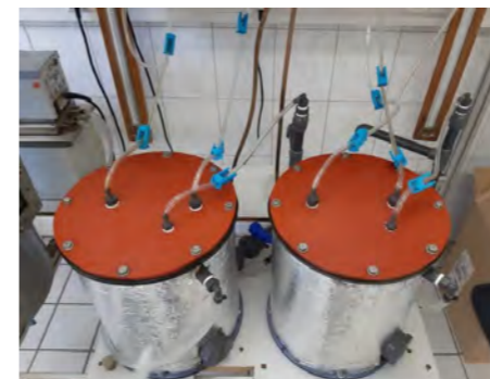
Fig.2: Up-flow fixed bed AD reactors
