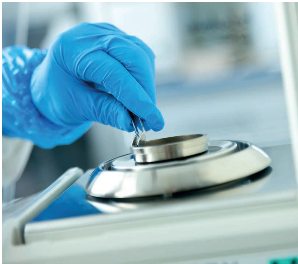
Fig. 41 Gravimetric measurement of dust load in the analytical lab
