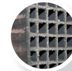
Application of mixed metal oxides alternatively to noble metal catalysts
