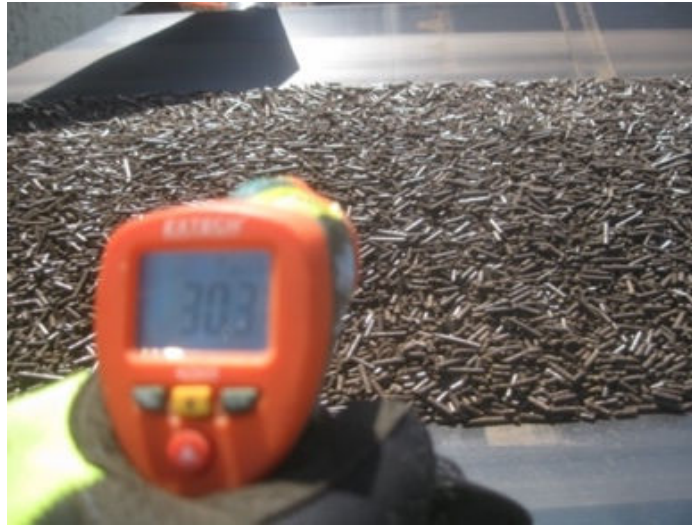
Figure 5: Checking for self-heating of torrefied pellets
