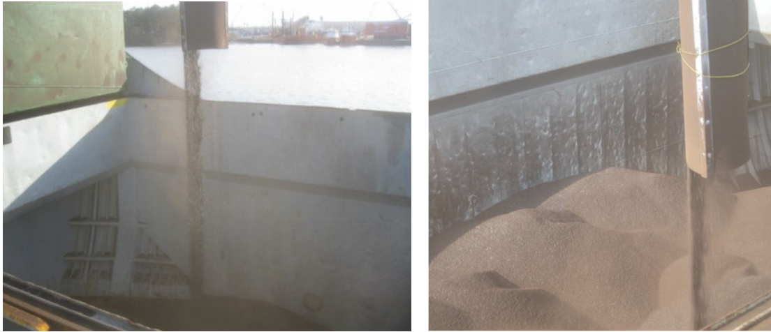
Figure 4: Loading torrefied pellets to MV Henny by New Biomass Energy in 2013. Although DU of pellets was above 98%, the unnecessary dropping height caused some breakage and dust which, different to white, beige or grey dust, becomes visible immediately. Pictures courtesy Carl Rheuban, New Biomass Energy LLC.
